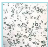
Fine, uniformly-sized spray droplets
